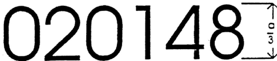
The ESA bearing the above EC type-approval mark is a device which has been approved in Germany (e1) under the base approval number 0148. The first two digits (02) indicate that the device conforms with the requirements of Directive 75/322/EEC, as amended by Directive  $\boxtimes$  2000/2/EC  $\boxtimes$ .
