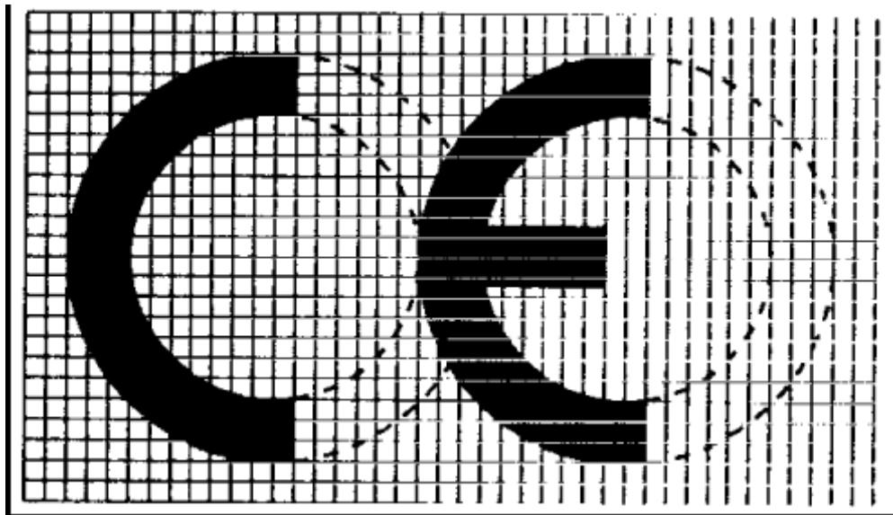
2. If the CE marking is reduced or enlarged the proportions given in the graduated drawing in paragraph 1 must be respected.
