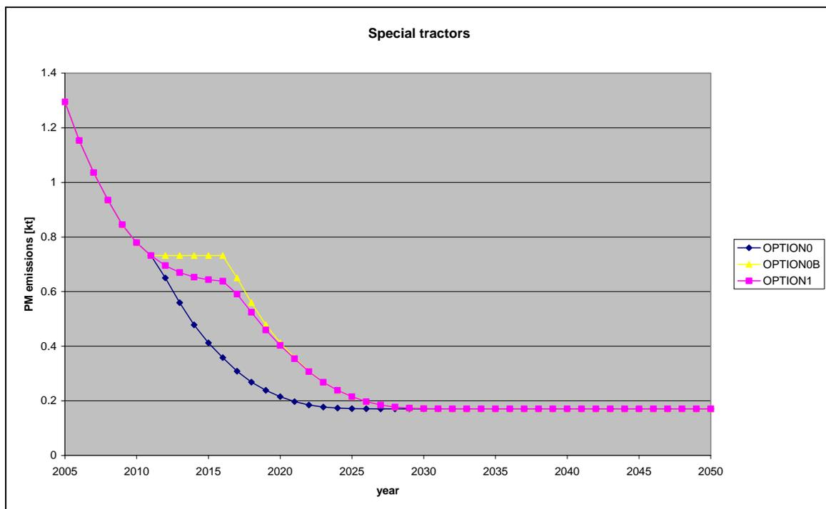
**Figure 3 PM emissions of Special agriculture tractors (time series 2005-2050)**
